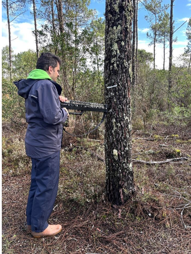
Figure IV-2. Slovenian collaborator Luka Krajnc measuring wood density with a resistograph on maritime pines in the Lacanau Genetic Conservation Unit. Source: A. Theraroz.
