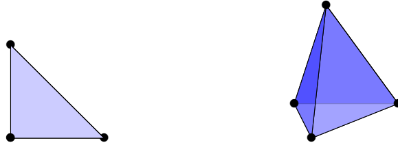
Figure 5 – Display of a triangle mesh element in 2D and tetrahedral mesh element in 3D.
