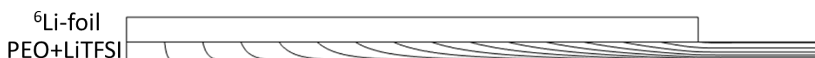
Figure IV-28. Schematic of the electric field lines simulated into the polymer electrolyte of the in-plane configuration.
