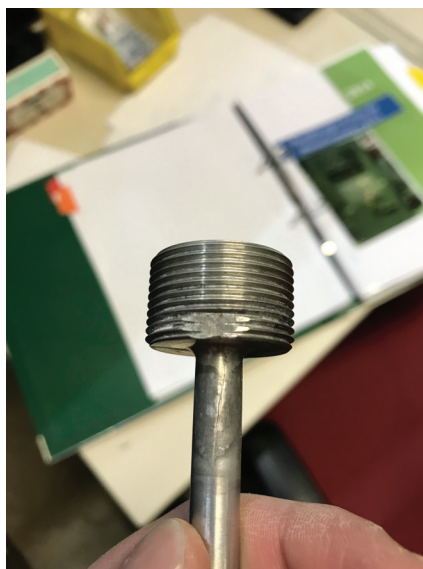
FIGURE 3.1 – High-Pressure cell after the breakage. Note the crack extending longitudinally from the threading.
