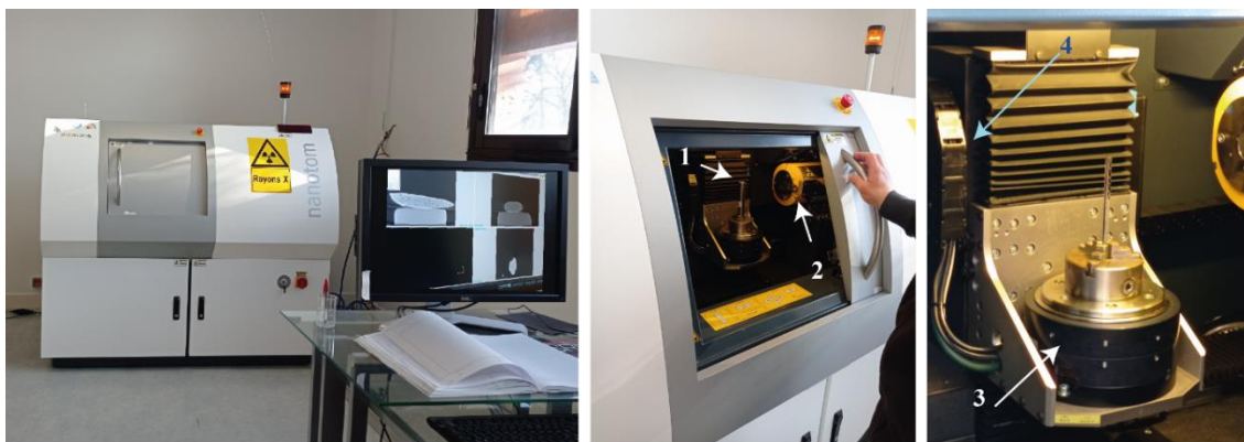
Figure 2.19. Nanotom Phoenix Micro-tomography. 1: Fibre rod with the sample adhered on the top; 2: source of X-ray; 3: rotating plate; 4: detector.
