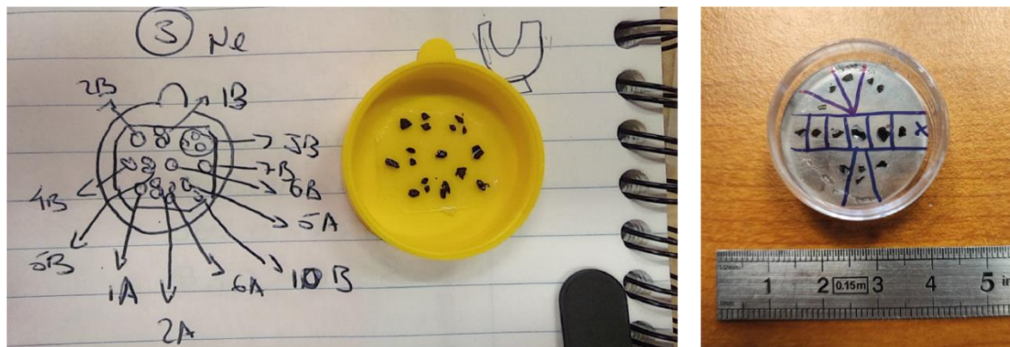
Figure 2.17. Example of epoxy before polishing (left) and ready for SEM and EMPA analysis (right).
