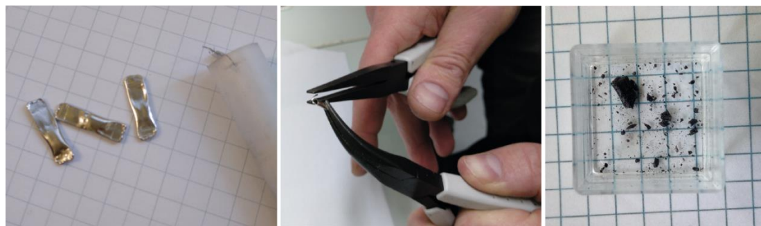
Figure 2.13. Resultant capsules after the experiment. As can be observed in the images, the preservation of the run product glass into a single piece is not easy due to the fragility of the glass (for the high vesicularity of it) and for the hardness of the capsule. The biggest pieces will be used for microtomography, and noble gases analysis. The tiniest pieces for SEM and EMPA, and the middles for FTIR.
