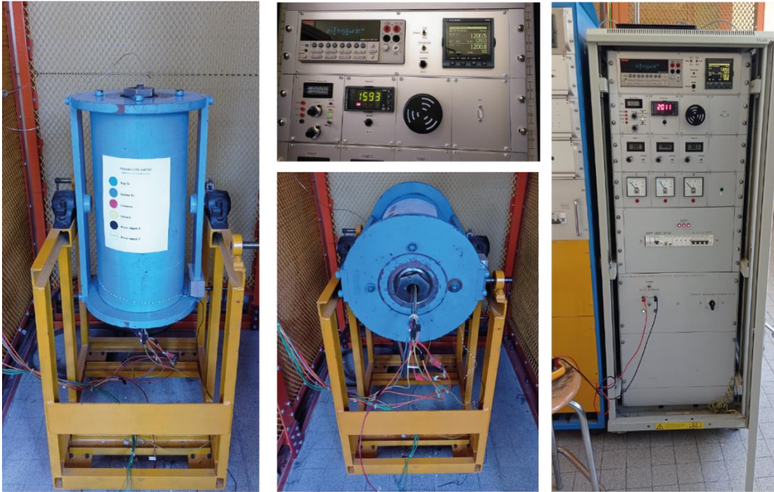
Figure 2.12. One of the autoclaves used to run the experiments. The upper part of the autoclave (left) is connected to the capillary that pressurize the experiment. In the lower part of the same image and the lower-middle image the connection exiting from the shutter and going to the controller (upper-middle and right image). The controller shows the conditions of two different experiments, while reaching the set-up conditions and while the experiment is running. In the right image, a voltmeter is controlling the quench connection. The small screen in the right shows the temperature if the upper and lower thermocouple and the screen in the middle part shows the pressure. The screen in the left allows us to control the intensity of the thermocouple's resistances.
