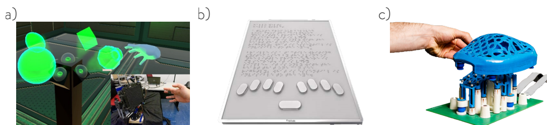
Figure 2.4 – a) PUMAH, mid-air interface [59]. b) Refreshable Blitab Braille tablet from Blitab Technology. c) HaptiComm device for tactile finger spelling designed by Duvernoy [34].
