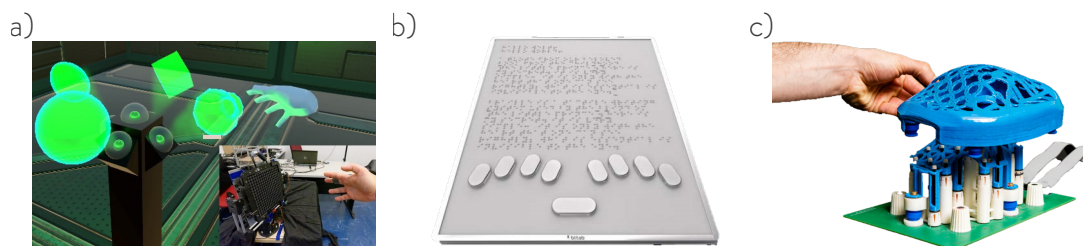
Figure 2.4 – a) PUMAH, mid-air interface [59]. b) Refreshable Blitab Braille tablet from Blitab Technology. c) HaptiComm device for tactile finger spelling designed by Duvernoy [34].
