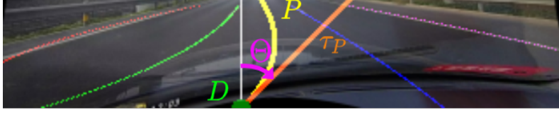
Figure 3.3: Visual servoing features computed by our development on real image.
