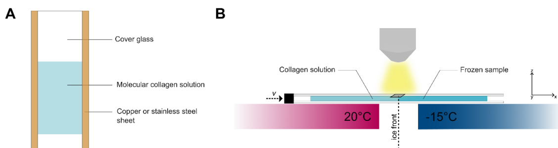
Figure 5. A) Experimental set-up of Hele-Shaw cells, comprising two thin sheets (200 \mu\text{m} ) of copper or stainless steel. Collagen solution at a concentration of 40 \text{mg}\cdot\text{mL}^{-1} was deposited in between two cover glasses, and the overall was sealed with a 100 \mu\text{m} -thick tape on the sides. B) The in situ cryoconfocal set-up enables to freeze the solution by imposing a controlled thermal gradient from 20 to -15^\circ\text{C} and follow the freezing front at the velocity of 10 \mu\text{m}\cdot\text{s}^{-1} .
