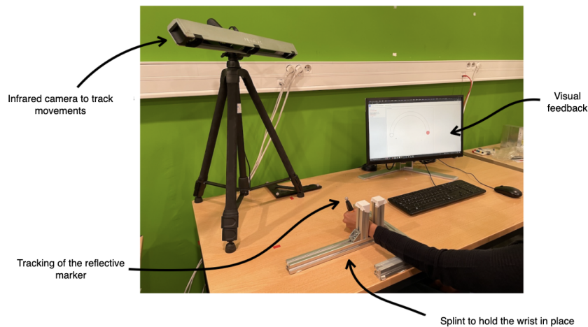
Fig. 3.3: Setup and apparatus used in the study. The participant’s forearm was placed in a splint. The participant traced a path using a marker, which was captured by an infrared camera. The marker controlled a cursor displayed on screen.
