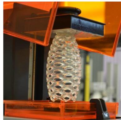
(d) 3D printed structure obtained by SLA process
