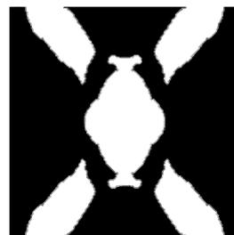
(b) Example of exotic material unit cell obtained by optimizing the elasticity tensor
