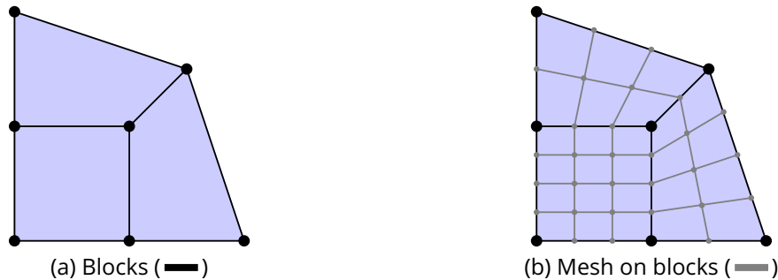
Figure 1.5: Blocking (a), and an example of mesh generated on this block structure (b).
