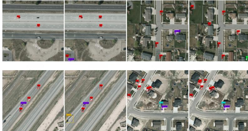
Figure 2.3 – Illustration of the detection results obtained with the YOLOD algorithm developed in (Luo et al., 2022). Red boxes are for detected cars. Purples boxes are for detected pickups. Orange boxes are for detected trucks. Cyan boxes are for detected boats. Green boxes are for detected camping cars.
