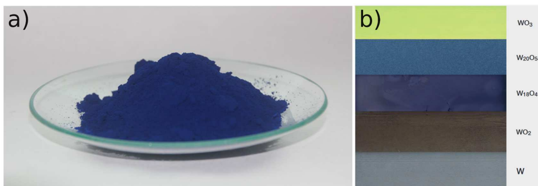
Figure 1.1 - (a) Prussian blue LUX pigment from Kremer Pigmente. Adapted from reference 12 . (b) Colors of various tungsten oxides and tungsten metal. Adapted from reference 13 .
