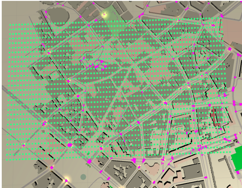
Figure 2.8: Three-dimensional environment model of Lille City 1 km 2 area with 2088 receiver grid represented in green squares.
