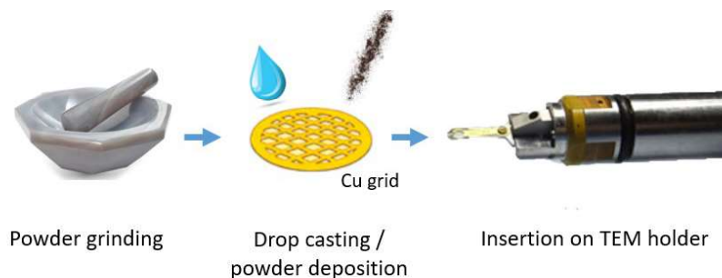
Figure 2.19: Steps of TEM powder sample preparation.
