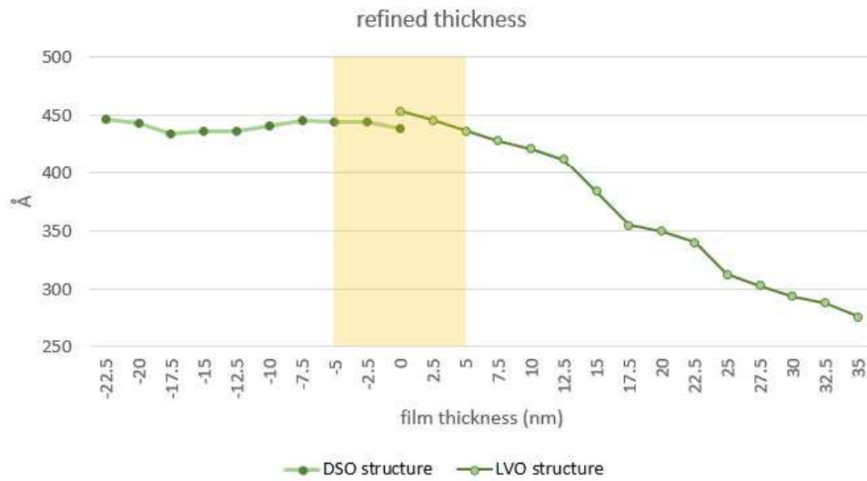
Figure 4.35: Refined thickness value for every ROI. The area around the interface where both the film and the substrate contribute to the diffraction patterns is highlighted in yellow.
