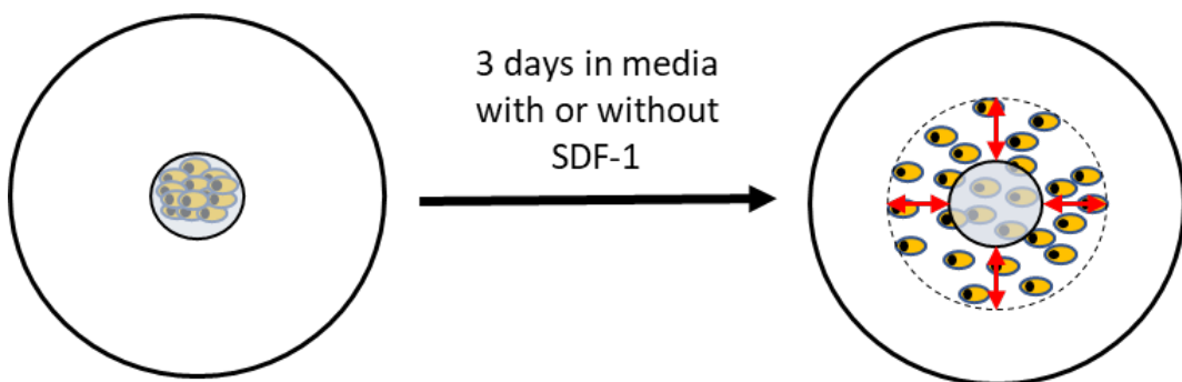
Figure 3. 2: Schematic representation of the agarose drop assay. A drop of cells in agarose is deposited in a well and covered with media with or without SDF-1 \alpha . After 3 days, the distance of migration is measured at 4 points (red arrows) as the distance from the edge of the drop to the edge of the migration front.
