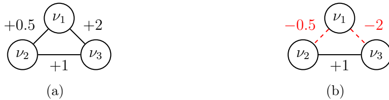
Figure 2.5: Example of two undirected graphs with three agents: (a) an undirected unsigned graph; (b) an undirected signed graph.
