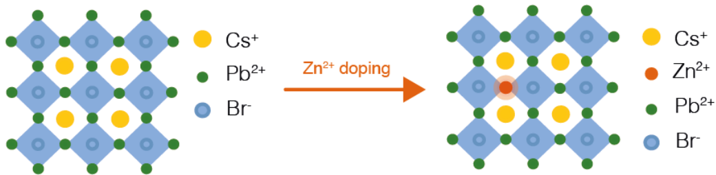
Fig. 5.1 Zn 2+ doping of CsPbBr 3 . Given the redox state of Zn, the Zn 2+ doping is likely to replace some Pb 2+ ions.
