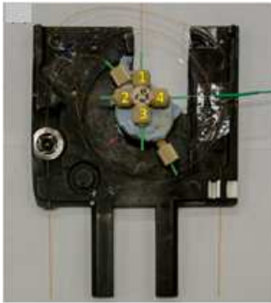
757 Fig. 3: CE-droplet microfluidics system for post-column detection: (A) schematic outline of 758 the setup used for postcolumn compartmentalization incorporated in a CE instrument. 759 The aqueous phase was segmented by oil in the tee connector (outside CE instrument) 760 and passed the separation capillary outlet to collect the electrophoresed effluent in a 761 compartmentalized manner (within CE instrument). (B) Photograph of the micro cross 762 as the droplet microfluidics interface was positioned in a capillary cassette. Photo 763 label: connection for (1) droplet capillary, (2) separation capillary, (3) detection 764 capillary, and (4) salt bridge electrode. (C) Separation of paralytic shellfish toxins 765 mixture: electropherogram from CZE-droplets microfluidics system demonstrating 766 separation and compartmentalization of electrophoresed analytes into preformed 767 droplets for oxidation. Reprinted from [39] with permission. Copyright (2014) Elsevier. 768
