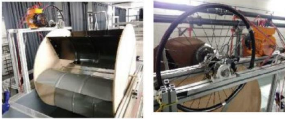
Figure 2.02: Reuse hydro turbine based on plywood, oil canister and bicycle wheel [55]
