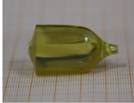
Figure III.26. A photograph of an as-grown Yb,Ho,Eu:CNGG crystal (11.5 at.% Yb 3+ , 1.25 at.% Ho 3+ , 0.075 at.% Eu 3+ ), the growth direction is along the [111] axis.
