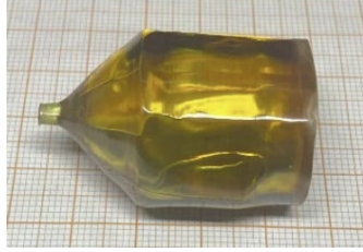
Figure V.1. As-grown Tm:LuVO 4 crystal boule, the growth direction is along the [001] axis.
