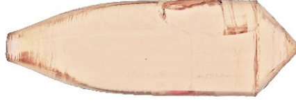
Figure III.1. An as-grown crystal boule, the growth direction is along the [100] axis.
