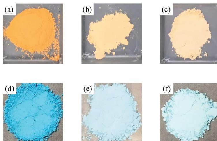
Figure 1.29. CaCO 3 with distinct colors produced through carbonation, with the introduction of dyes; (a), (b), (c): Sunset Yellow FCF, with citric acid aqueous solution additions of 0 cm 3 , 5 cm 3 , and 8 cm 3 , respectively; (d), (e), (f): Brilliant Blue FCF, with citric acid aqueous solution additions of 0 cm 3 , 5 cm 3 , and 8 cm 3 , respectively.
