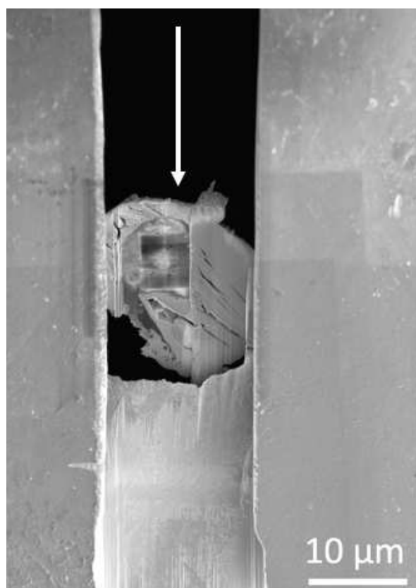
Figure 2.28. CaCO 3 +naphthazarin section (white arrow) prepared for STEM-EELS using FIB-SEM.
