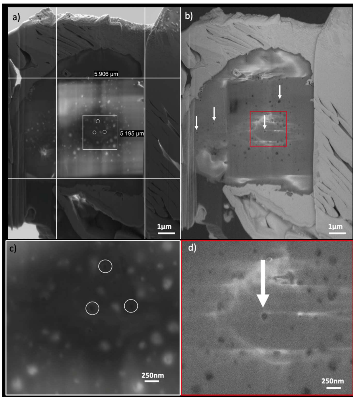
Figure 4.21. SEM micrographs of the FIB lamella section of calcite+0.53 mM naphthazarin of 60-70 nm thickness a), c) SE detector, b), d) ESB detector. c) and d) are zoomed-in views of an area on micrograph (a) and micrograph (c) respectively.
