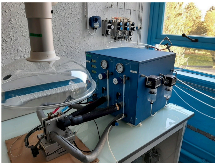
Figure II - 1 - 1: Picture of the Fuel Cell Test Station FCT-150S from Biologic, connected to the home-made gas network.
