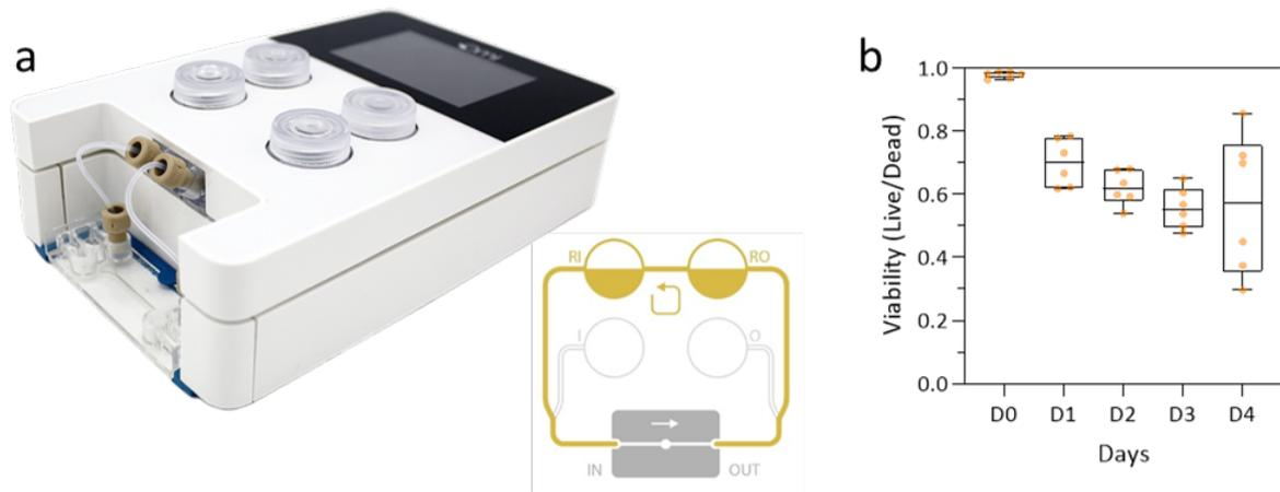
**Figure 4.6** – Recirculation using Omi device (Fluigent). (a) Device and reservoirs layout. (b) Viability of MDA-MB-231 cells recirculated with Omi through a control chip (BE-Flow Standard from BEOnChip, straight channel of  $375\ \mu\text{m}$  height) for 5 days.
