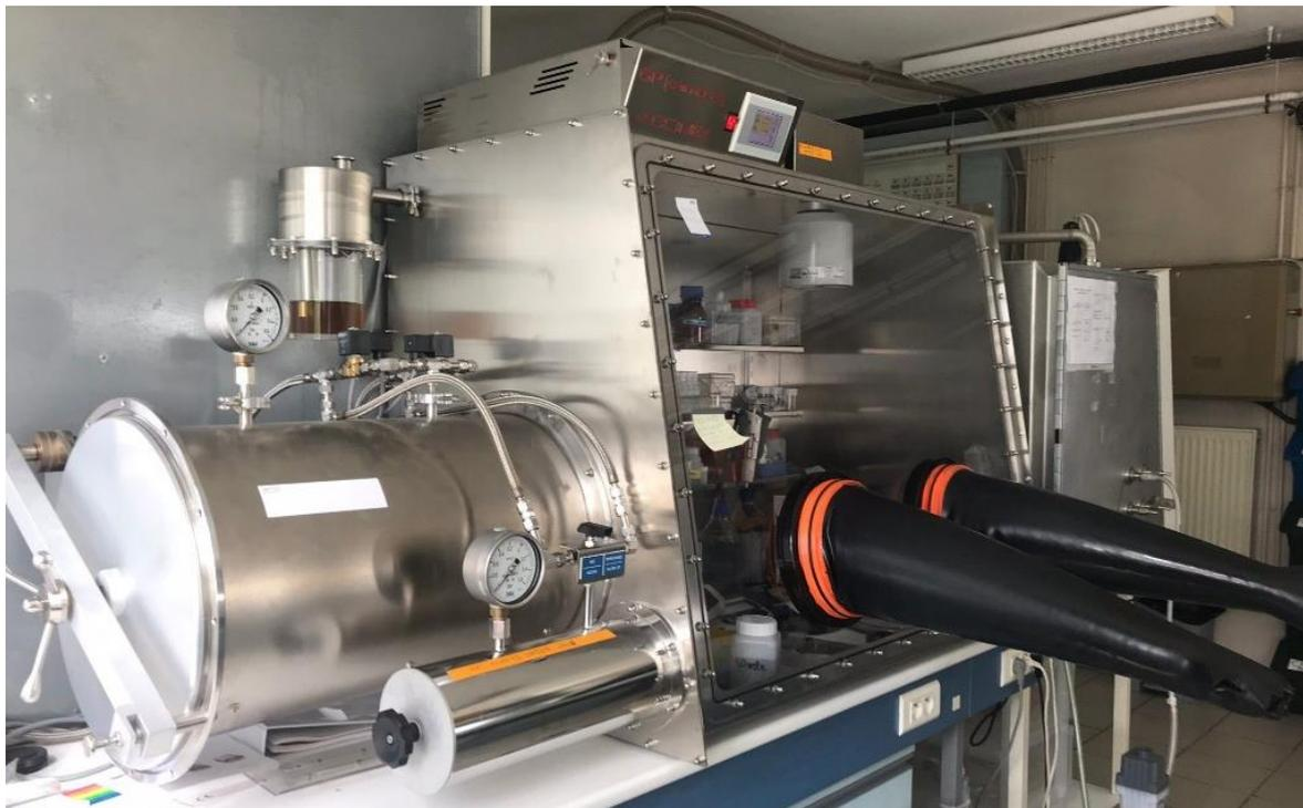
*Figure 3.2.1.1. A wet glove-box used for synthesis, conditioning, and storing C-S-H samples at the geochemistry laboratory, ISTerre.*
