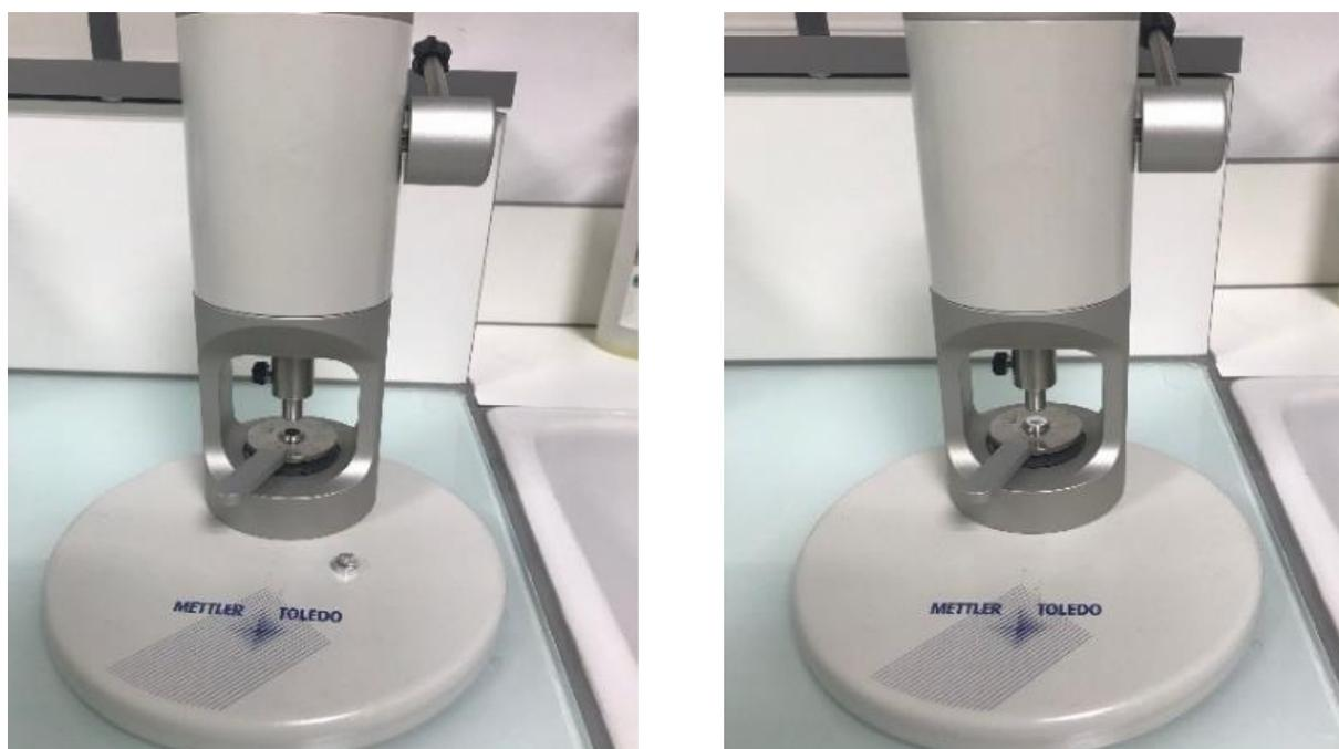
Figure 3.2.4.1. (left) Sealing press for Al crucibles for thermogravimetric analysis with Al cell and a cap (right) after the crucible was sealed.
