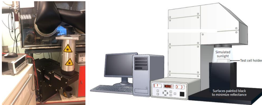
Figure 1.3 : The solar simulator in our STEP lab connected to a Keithley digital source meter.
