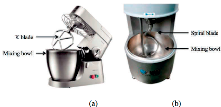
Figure III.2.1.1. Mechanical low shear mixers Kenwood Major 1200 (Kenwood, United Kingdom) equipped with a K blade (a) and SPI10 (VMI, France) equipped with a spiral blade (b)
