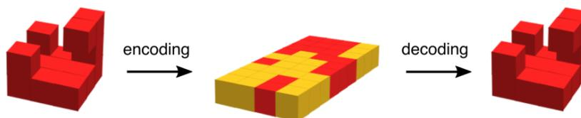
Figure 3.36: The method of shape replication used in [7]. Here, the initial shape is an assembly that may have to be destroyed in the process.
