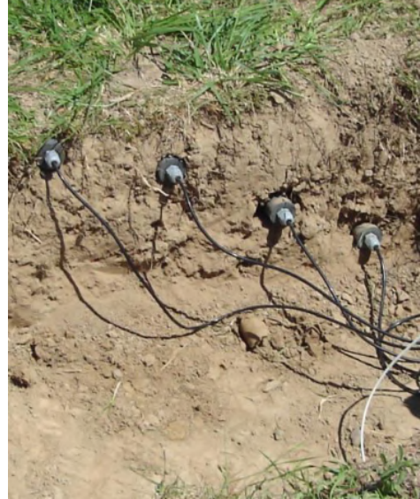
Figure 1.10: FDR probes (Tethaprobos) installed at depths of 5 cm, 10 cm, 20 cm and 30 cm in the SMOSMANIA Montaut site. Picture from the supplement of Calvet et al. [2016].
