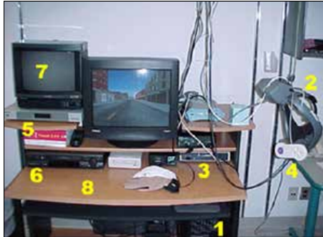
1. ZX-10 Intergraph Computer Workstation. 2. Proview XL-50 Mounted Display. 3. miniBird 800 6 Degree-of-Freedom tracker. 4. Joystick. 5. Sony Scan Converter. 6. Mitsubishi Video Cassette Recorder. 7. Sony TV monitor. 8. Movable desk unit.
