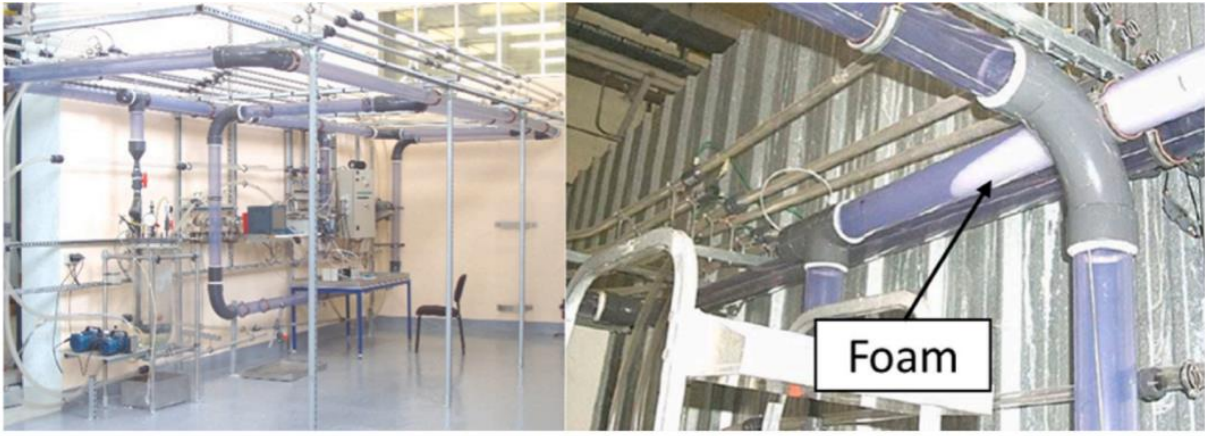
Figure 1.5.5. Pictures of the pilot set up used for the study of foam flow for nuclear decontamination. The figure was adapted from (Gossard et al., 2022).
