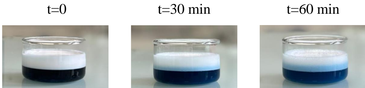
Figure S7: Photographs of the imbibition test at different times. The aqueous phase containing a blue dye is entering inside the foam with time showing the imbibition process of the foam. The foam corresponds to the one of 27% of liquid fraction.
