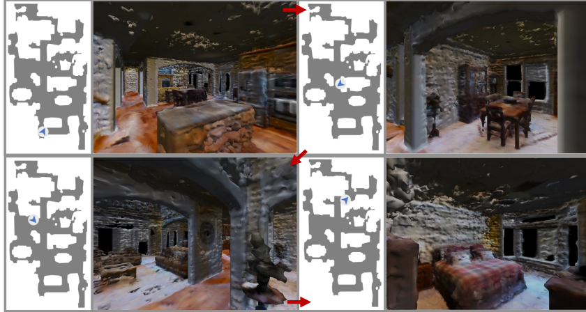
Figure 6.5: Navigating in the Habitat simulator: The underlying mesh was extracted from the trained NeRF, Ours (cov) . Rendering quality and the generated BEV map are correct, as are free navigable space and collision handling. Temporal order indicated by \rightarrow .
