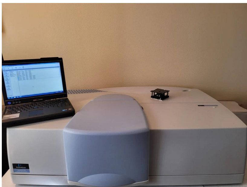
Fig 2.4 The Perkin Elmer Lambda 950 High-Performance UV/Vis/NIR Spectrophotometer
