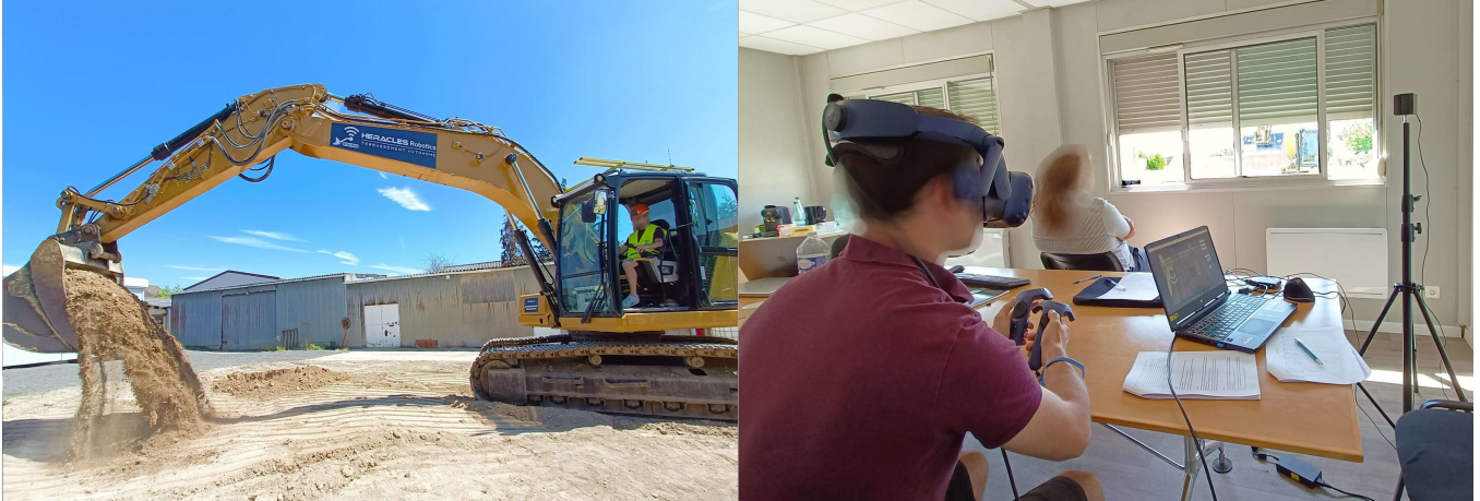
Figure 6.3: Interface Comparison Setup Example - Real Machine (Left) versus VR Interface Remote Control (Right)
