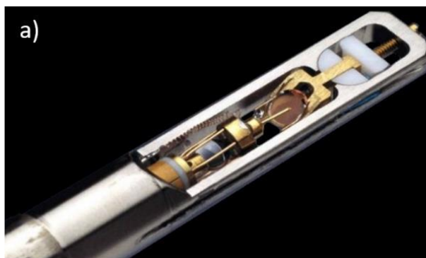
Figure 2.2: Photo of the Nanofactory sample holder used for in situ TEM measurements. Reproduced from Villepreux's PhD thesis [72].
