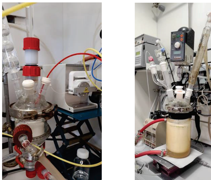
Figure VIII-3: 75 mL (left) and 1000 mL (right) glass reactors with the pump to feed the TBHP solution.
