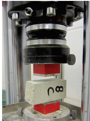
Figure VI-14: Picture of the compressive test carried out on a half prism with the MTS Systems multifunction press.
