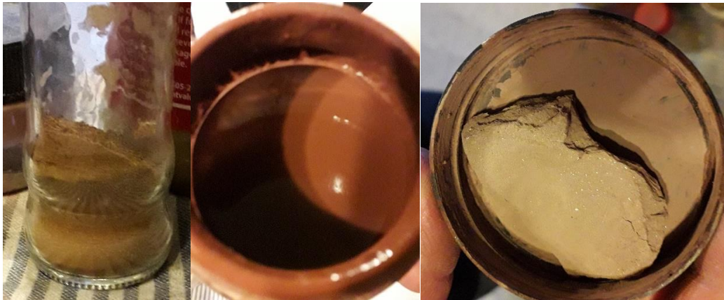
Figure 83: From left to right: Hematite powder which becomes dark when fired, manganese, and mica (my photos)
