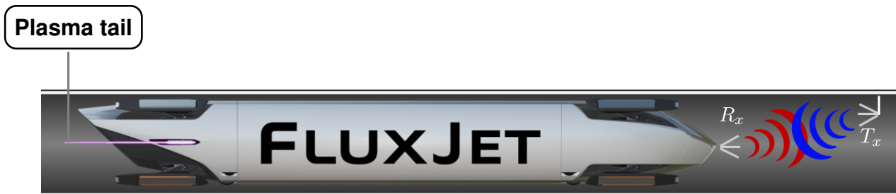
Figure 3.18: Schematic of the TransPod system with the plasma-based power transmission system and transmitter/receiver inside the steel tube.
