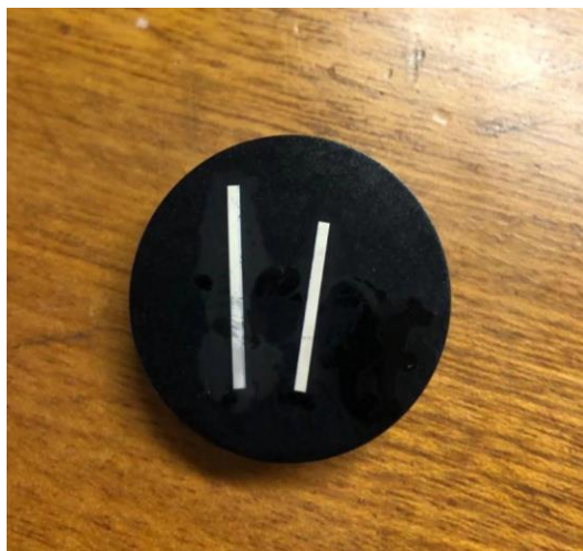
Figure II-4. Samples prepared for indentation test.
