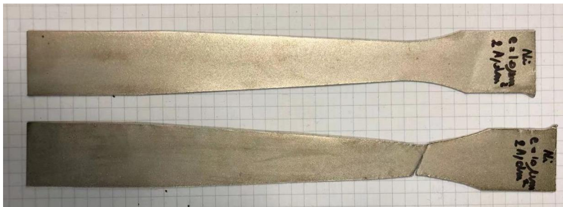
Figure III-20. Specimen pure Ni coated before and after tensile test.
