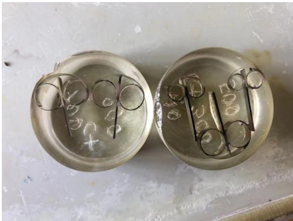
Figure A-1. An example of the well-prepared metallic etching specimens.
