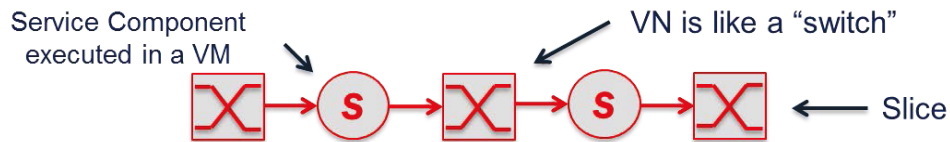
Figure 1 – Example: a service made of a number of service components (S) executed on Virtual Machines (VM) interconnected via Virtual Network (VN)
