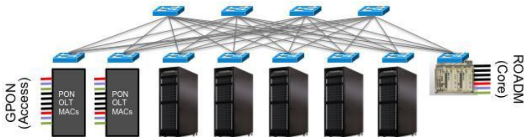
Figure 8 - Target hardware, constructed from commodity servers, storage, and switches [9].
