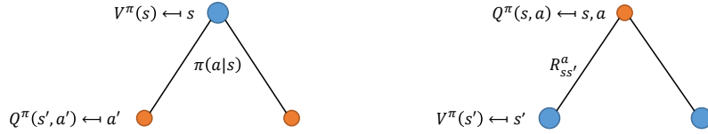
Figure 2.7: Relationship between the value function and the Q-function.
