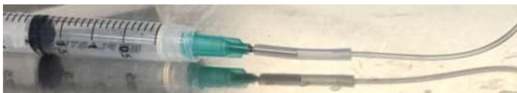
Figure 29: Connection system: 18G blunt-end Luer lock syringe needle (Darwin fz13) connected to a “Novosil” silicone tube of internal diameter 1 mm (Fisher Scientific®). This system allowed connecting a syringe to a flexible plastic tubing (Tygon®) of internal diameter 0.5 mm, which fitted perfectly inside the inlet/outlet punch
