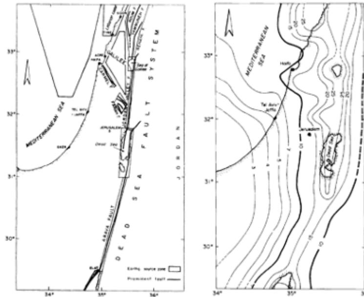
Fig. 2. 6 (a) Source model used for the seismic hazard calculation, (b) Hazard maps for the PGA at 475 years return period (from Arieh et al. 1989)
