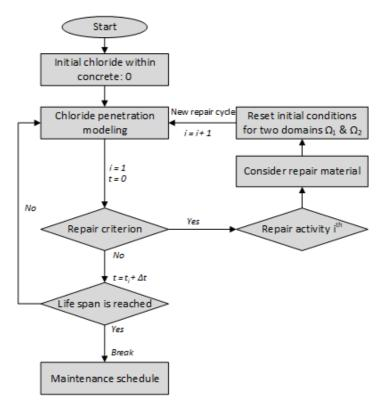
Figure 2.8: Modeling process of chloride ingress in repaired concrete
