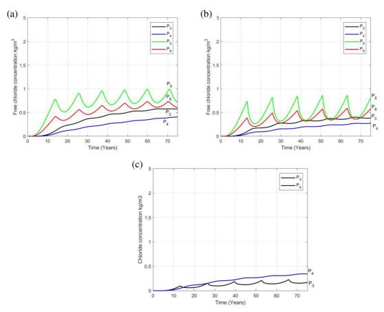
Figure 2.19: The evolution of chloride concentration in different locations of unrepaired, aged concrete (a) OCR1, (b) OCR2, (c) CCR3
