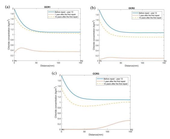
Figure 2.17. The chloride concentration at the depth of concrete cover (a) OCR1, (b) OCR2 (c) CCR3
