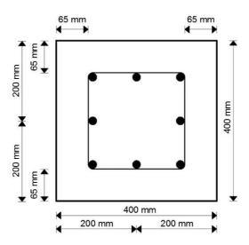
Figure 3.13 : Cross-sectional of square column
