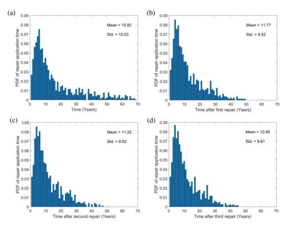
**Figure 3.2:** PDF of repair application time (a) First repair application (b) Second repair application (c) Third repair application (d) Fourth repair application
