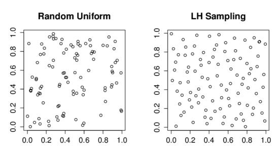
Figure A.1: Comparison between random sampling and LHS
