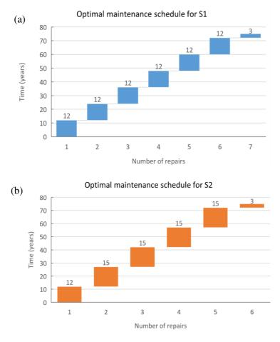
Figure 3.18: Optimal maintenance schedule for (a) S1, (b) S2
