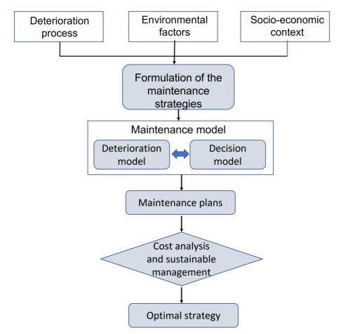
Figure 1.2: Conceptual framework of a management system
