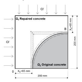
Figure 4.5: Circular concrete replacement method with S1 and S2 repair options
