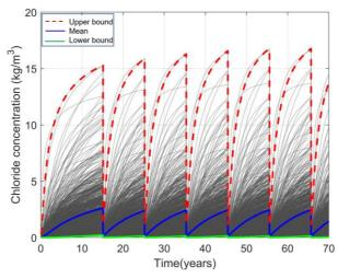
Figure 3.4: Time-dependent chloride concentration profiles at rebar cover
