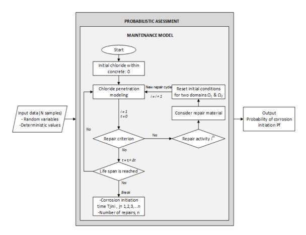
Figure 3.1. Flow chart of probabilistic maintenance modeling
