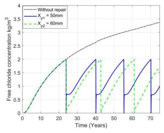
Figure 2.10: Time-dependent evolution chloride concentration at the cover depth without and with repair
