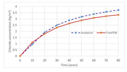
Figure 2.3: Model validation for one-dimensional chloride ingress
