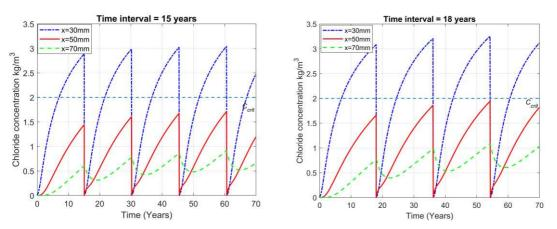
**Figure 2.12:** Time-dependent evolution of the chloride concentration at three depths (x = 30, 50 and 70 mm) with  $X_p = 60$  mm and (a) 15-year repair interval, or (b) 18-year repair interval
