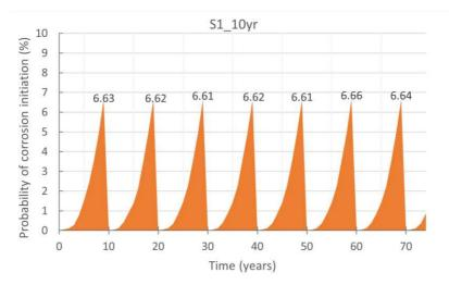
Figure 3.16: Probability of corrosion initiation for S1-10yr repair strategy
