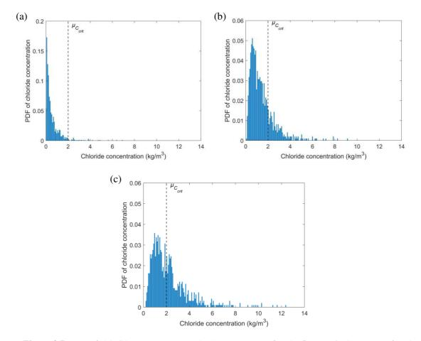
**Figure 3.7:** PDF of chloride content at cover depth (a) one year after the first repair (b) 5 years after the first repair (c) 10 years after the first repair
