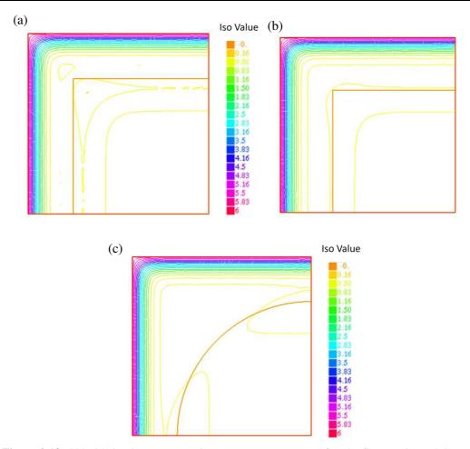
Figure 2.18: Chloride ion iso-concentration contours at one year after the first repair (a) OCR1, (b) OCR2 (c) CCR3
