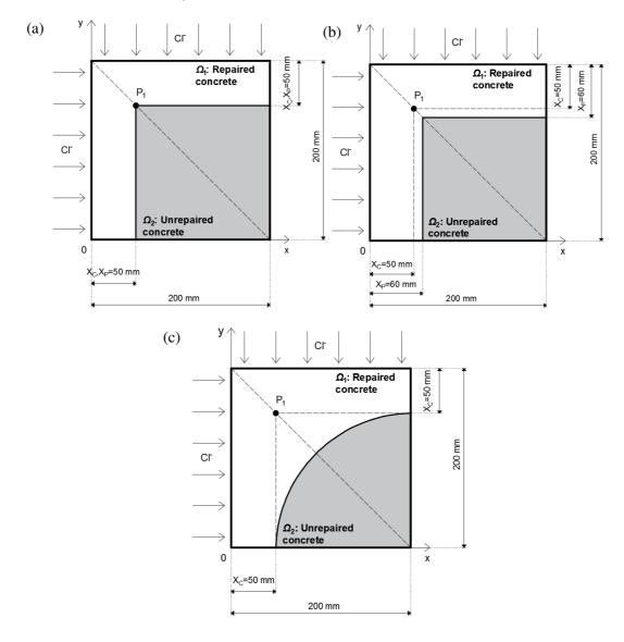
Figure 4.4: Three repair strategies (a) OCR1 with  $X_p = X_c$ , (b) OCR2 with  $X_p > X_c$  (c) CCR3
