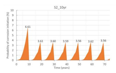
Figure 3.17: Probability of corrosion initiation for S2-10yr repair strategy
