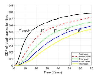
Figure 3.3: CDF of repair application time
