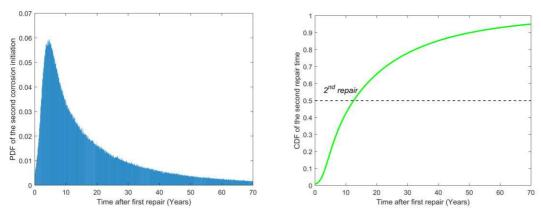
Figure 3.11: PDF and CDF of the second repair time
