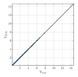
Figure 3.12: Comparison of maintenance model ( $Y_{true}$ ) and PCE model ( $Y_{PCE}$ ) for the chloride concentration at critical depth at Y15 (400 samples)
