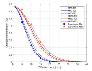
Figure 2.4: Chloride diffusion model validation with data taken from (Yu et al., 2021)
