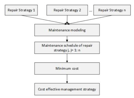
Figure 4.1: Framework for cost comparison of different repair strategies
