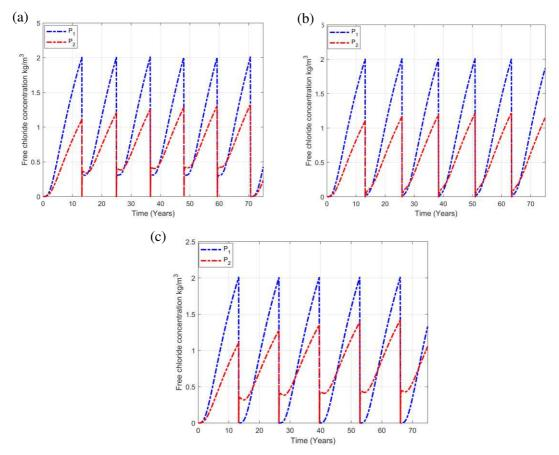
**Figure 2.15**: The evolution of chloride concentration in different locations of repair concrete (a) OCR1, (b) OCR2 (c) CCR3
