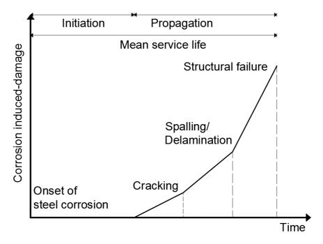
Figure 1.1: The corrosion process of RC structures
