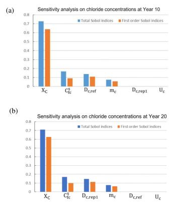
Figure 3.19: Influences of input parameters on chloride concentration at (a) year 10 (before repair) and year 20 (after repair)
