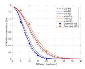
Figure 3: Chloride diffusion model validation with data taken from (Yu et al., 2021)
