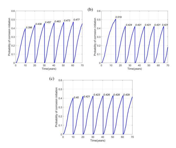
**Figure 3.8:** Probability of corrosion initiation of two cases (a) 10-year repair intervals (b) 20mm extra replacement depth (c) 10-year repair intervals and 20 mm extra replacement depth
