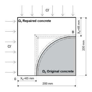
Figure 3.14: Circular concrete replacement method
