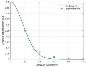
Figure 2.5: Chloride diffusion model validation with data taken from (Roy, Liam Kok Chye and Northwood, 1993)
