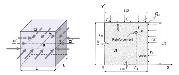
**Figure 2.1**: (a) 2D chloride ingress area of concrete to be modeled, (b) Boundary conditions of a truncated chloride ingress model
