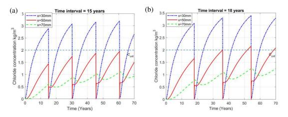
**Figure 2.11.** Time-dependent evolution of the chloride concentration at three depths (x = 30, 50 and 70 mm) with  $X_p = 50$  mm and (a) 15-year repair interval, or (b) 18-year repair interval
