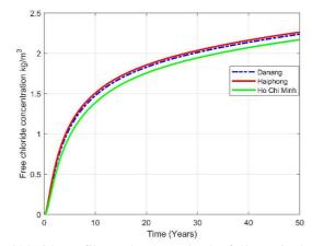
Figure 2.20: Chloride profiles at the cover depth of 50 mm in three coastal cities
