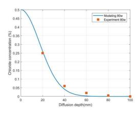
Figure 4: Chloride diffusion model validation with data taken from (Roy, Liam Kok Chye and Northwood, 1993)
