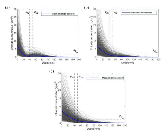
**Figure 3.6:** Chloride profiles (a) one year after the first repair (b) 5 years after the first repair (c) 10 years after the first repair
