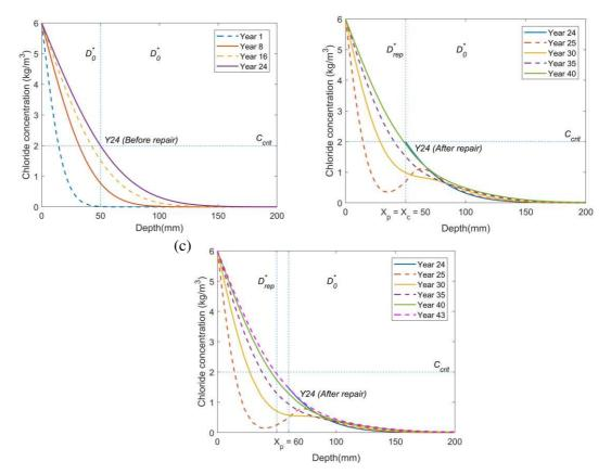
Figure 2.9: Chloride profiles: (a) before repair, (b) after repair with  $X_{p1}$ , (c) after repair with  $X_{p2}$
