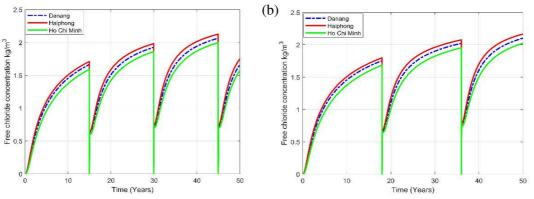
Figure 2.21: Chloride profiles with repair interval of (a) 15 years, (b) 18 years (50 mm concrete replacement depth  $X_p = 50$  mm)
