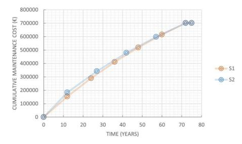
Figure 4.6: Cumulative maintenance cost of each repair strategy S1 and S2
