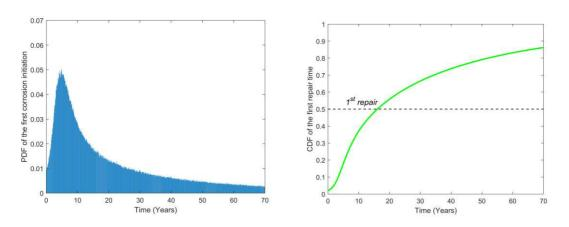
Figure 3.10: PDF and CDF of the first repair time
