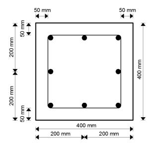
Figure 2.13: Cross-sectional of square column
