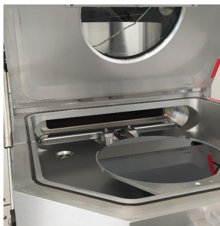
Figure 2: Open chamber corresponding with the load lock. This photography was acquired during a maintenance operation under atmospheric conditions. In working conditions, this opening only occurs when vacuum equilibrium is reached between deposition chamber and load lock.
