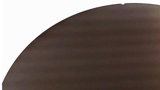
Figure 18 : Photo of pp(V3D3) deposition on a silicon wafer, showing the appearance of lines following the plasma torch's movement pattern.
