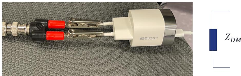
Figure D-4 DM impedance measurement and the model of the phone charger.
