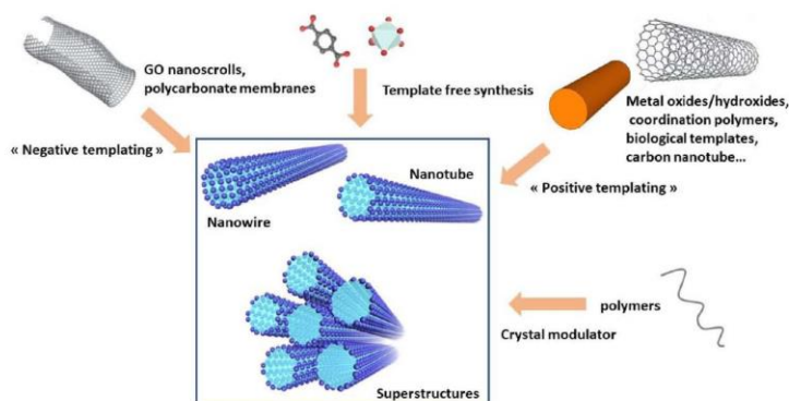
Figure 1. Schematic illustrations of the different strategies used to prepare tubular MOF-based nanostructures and superstructures.
