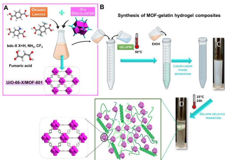
Figure 1. Schematic drawing of (A) room-temperature synthesis of UiO-66-X ( X = \text{H}, \text{NH}_2, (\text{CF}_3)_2 ) and MOF-801, (B) synthesis approach of the UiO-66-X ( X = \text{H}, \text{NH}_2, (\text{CF}_3)_2 )/gelatin and MOF-801/gelatin composites. (C,D) Photographs of UiO-66/gelatin hydrogels obtained just after the addition of ethanol (C) and after aging at RT for 24 h (D). Zr polyhedral, carbon, oxygen, nitrogen, fluoride, and hydrogen are in pink, gray, red, blue, green, and white, respectively.
