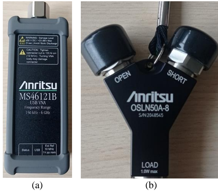
Figure 3.11 (a) Compact 1-port vector network analyzer Anritsu® MS46121B (150 kHz – 6GHz). (b) Calibration-kit Anritsu® (OSLN50A-8).
